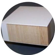
**End Grain Balsa** provides superior strength, and is recognized as one of the most versatile core materials for sandwich construction. This closed cell material is non-absorptive, and extremely strong with an 11 lb. density rating. Balsa is also an environmentally friendly, ecological resource core material.
